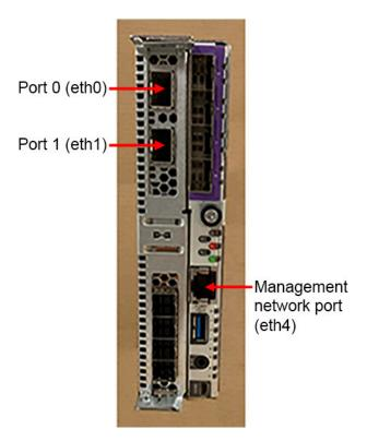
The figure below shows the locations of the Ethernet ports on a server module that has a 10GBase-T Ethernet PCle card installed in it.
