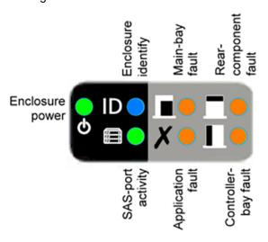
The figure below shows the front LEDs and icons on an expansion enclosure.
