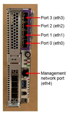
The figure below shows the locations of the Ethernet ports on a server module that has a 25Gb Ethernet SFP28 PCIe card installed in it.
