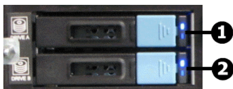
Figure 11 Hard disk drives status and activity status LEDs - models 4060, 4080, and 4100
