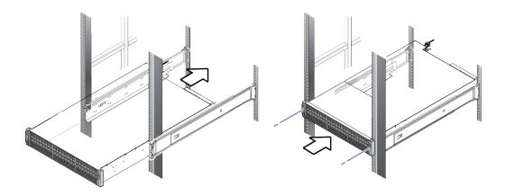
**9.** Find the washers, O-rings, and screws included with the bezel bracket mounting kit (part number 043-100885-01.P). Then install a washer, O-ring, and screw (one per side) between the mounting profile of the rack and the mounting "ears" of the controller. The screw engages the threaded hole in the rail.
