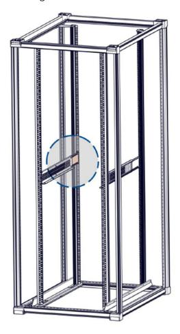
**5.** Use two flathead screws to secure the rails to the rear vertical post on the rack.
