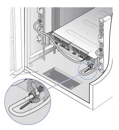
**4.** Connect the PDUs to separate external power sources on different branch circuits.
