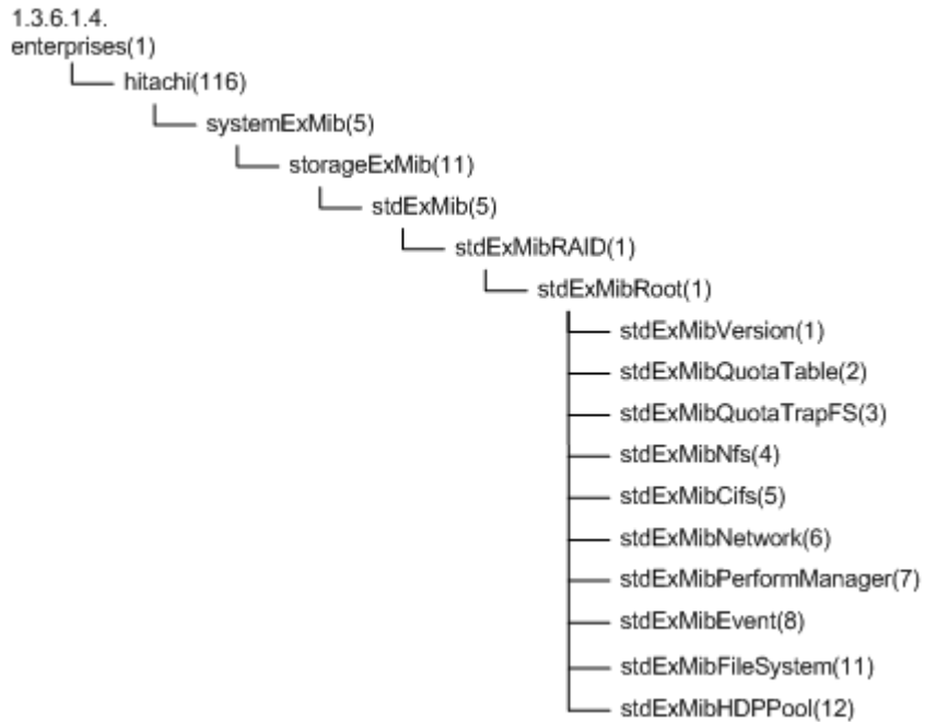
Figure G-2 Groups of MIB objects for responding to SNMP get requests and tables to be referenced (standard MIB objects)
