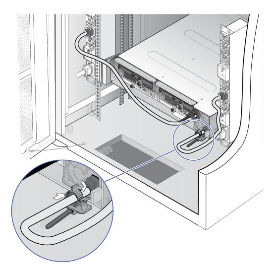
**4.** Connect the PDUs to separate external power sources on different branch circuits.
