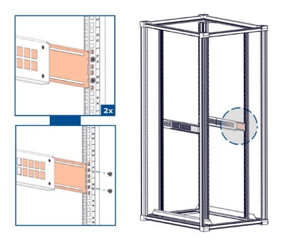
**6.** Tighten the four screws on the left mounting rail.
