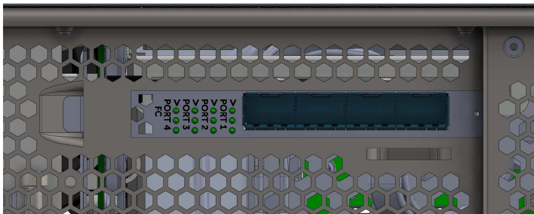
Figure 9 Fibre Channel storage ports label
