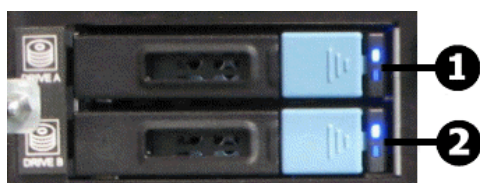
Figure 8 Hard disk drives status and activity status LEDs - models 4060, 4080, and 4100
