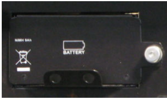
Figure 7 Model 4060, 4080, and 4100 NVRAM backup battery pack (front view)
