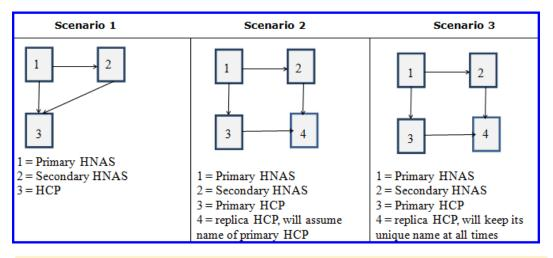
**Caution:** Care should be taken when configuring systems with a single migration destination for both replication source and target (known as a triangular arrangement). Such arrangements should not be considered a valid solution in any disaster recovery (DR) or backup scenario, as there is only a single copy of the user data pointed to by XVLs at each end of the replication policy.
