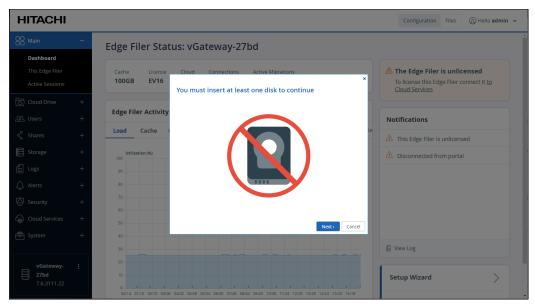
Add a disk to the HCP Anywhere Enterprise Edge Filer virtual machine. Otherwise, the **Name this Edge Filer** window is displayed.
