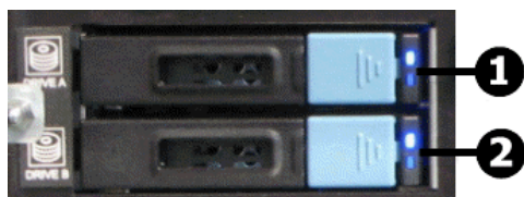
Figure 12 Hard disk drives status and activity status LEDs - models 4060, 4080, and 4100
