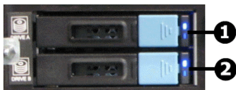
Figure 12 Hard disk drives status and activity status LEDs - models 4060, 4080, and 4100
