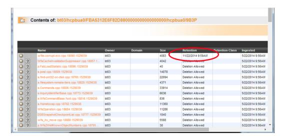
The HCP Disposition service periodically runs to delete files for which the retention period has expired so that they do not remain permanently on HCP.
