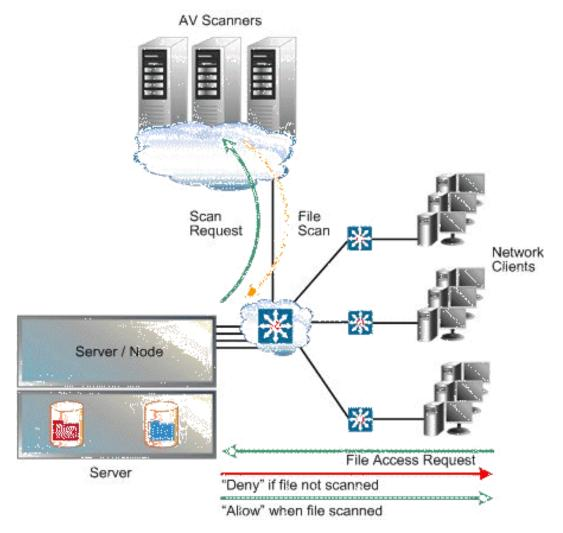
You can configure multiple Virus Scan Engines to enhance both the performance and to maintain high-availability of the server. If a Virus Scan Engine fails during a virus scan, the storage server automatically redirects the scan to another Virus Scan Engine.
