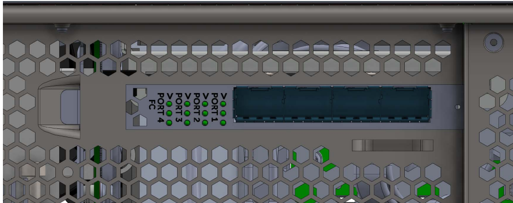
Figure 9 Fibre Channel storage ports label
