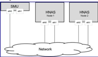
The first figure displays a single node network configuration and the second a clustered network configuration. Each node requires two IP addresses:
