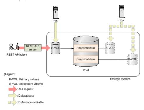
To store snapshot data, create a Thin Image pair where an LDEV or a DP volume is used as a primary volume, and a virtual volume for Thin Image or a DP volume is used as a secondary volume. If the created pair is registered to a snapshot group or a consistency group, processing can be performed by group. If a consistency group is defined, the snapshot data from when the storage system received a request can be stored for all the primary volumes in that consistency group.
