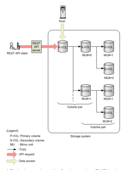
A ShadowImage pair consists of a primary volume (P-VOL) and a secondary volume (S-VOL). The primary volume can be paired with more than one secondary volume. Each secondary volume is managed according to the MU (mirror unit) number.
