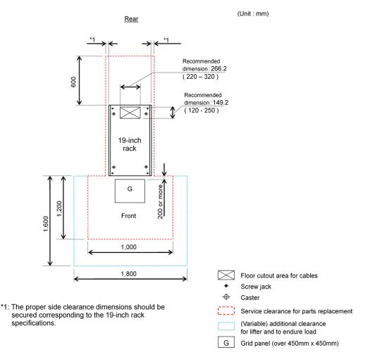
If your computer room uses floor cutouts to route power and data cables, position the cutouts toward the center of the rack. If this is not possible, position the cutouts off-center from the rack as long as the cutout is within the allowable range and allows smooth routing and entrance of cables. Check the relationship between the position of the cutout and the cable openings on the rack.
