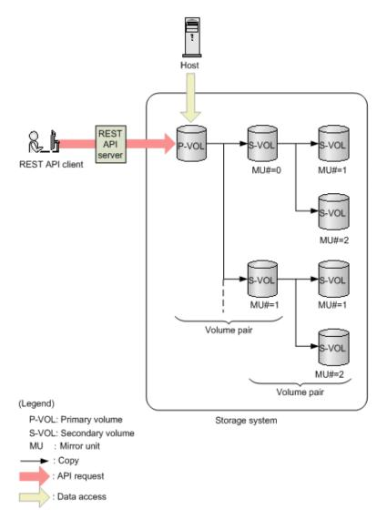
A Shadowlmage pair consists of a primary volume (P-VOL) and a secondary volume (S-VOL). The primary volume can be paired with more than one secondary volume. Each secondary volume is managed according to the MU (mirror unit) number.
