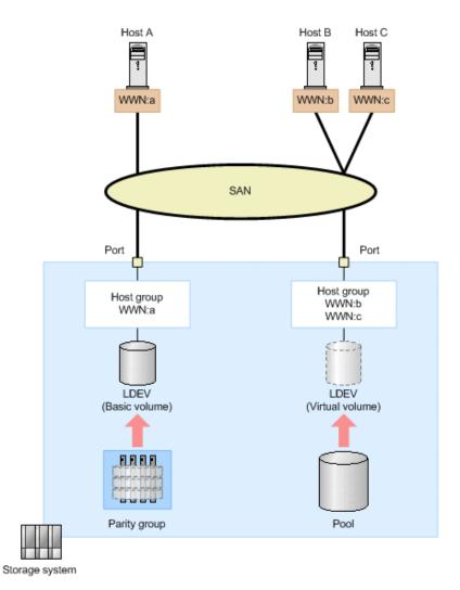
In the preceding figure, an LDEV is created from the parity group, and the LU path is set for the host group in which the WWN of host A is registered. In addition, another LDEV is created from the DP pool, and the LU path is set for the host group in which the WWNs of host B and host C are registered. By registering the WWNs of multiple hosts in the host group, you can apply the same settings for accessing the LDEV to the hosts at the same time.
