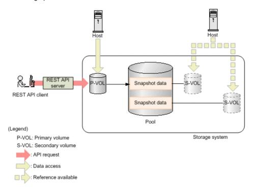
To store snapshot data, create a Thin Image pair where an LDEV or a DP volume is used as a primary volume, and a virtual volume for Thin Image or a DP volume is used as a secondary volume. If the created pair is registered to a snapshot group or a consistency group, processing can be performed by group. If a consistency group is defined, the snapshot data from when the storage system received a request can be stored for all the primary volumes in that consistency group.
