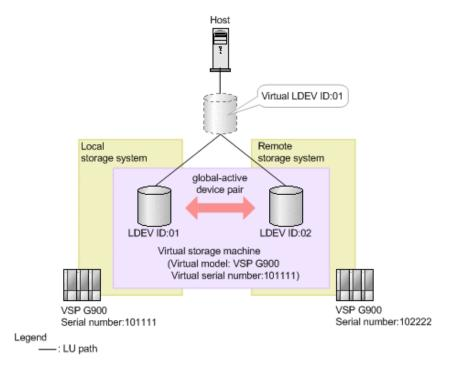
If you issue an API request from a REST API client, you can create a global-active device pair, or perform operations on pairs when stopping either storage system for maintenance.
