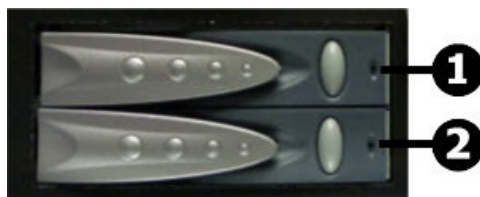
Figure 5 Hard disk drives status and activity status LEDs - models 3080 and 3090
